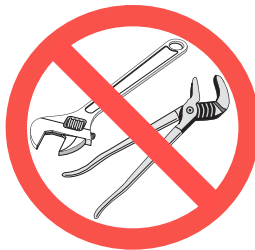
Figure 4-1. Do Not Use Pliers or Adjustable Wrenches
